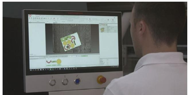
The SVS, acronym for Sheet/Scrap Vision System, helps to re-use sheet metal leftovers
